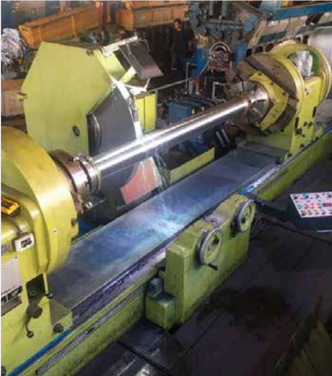
Piston Rod Reconditioning by SAW or by Laser Cladding
