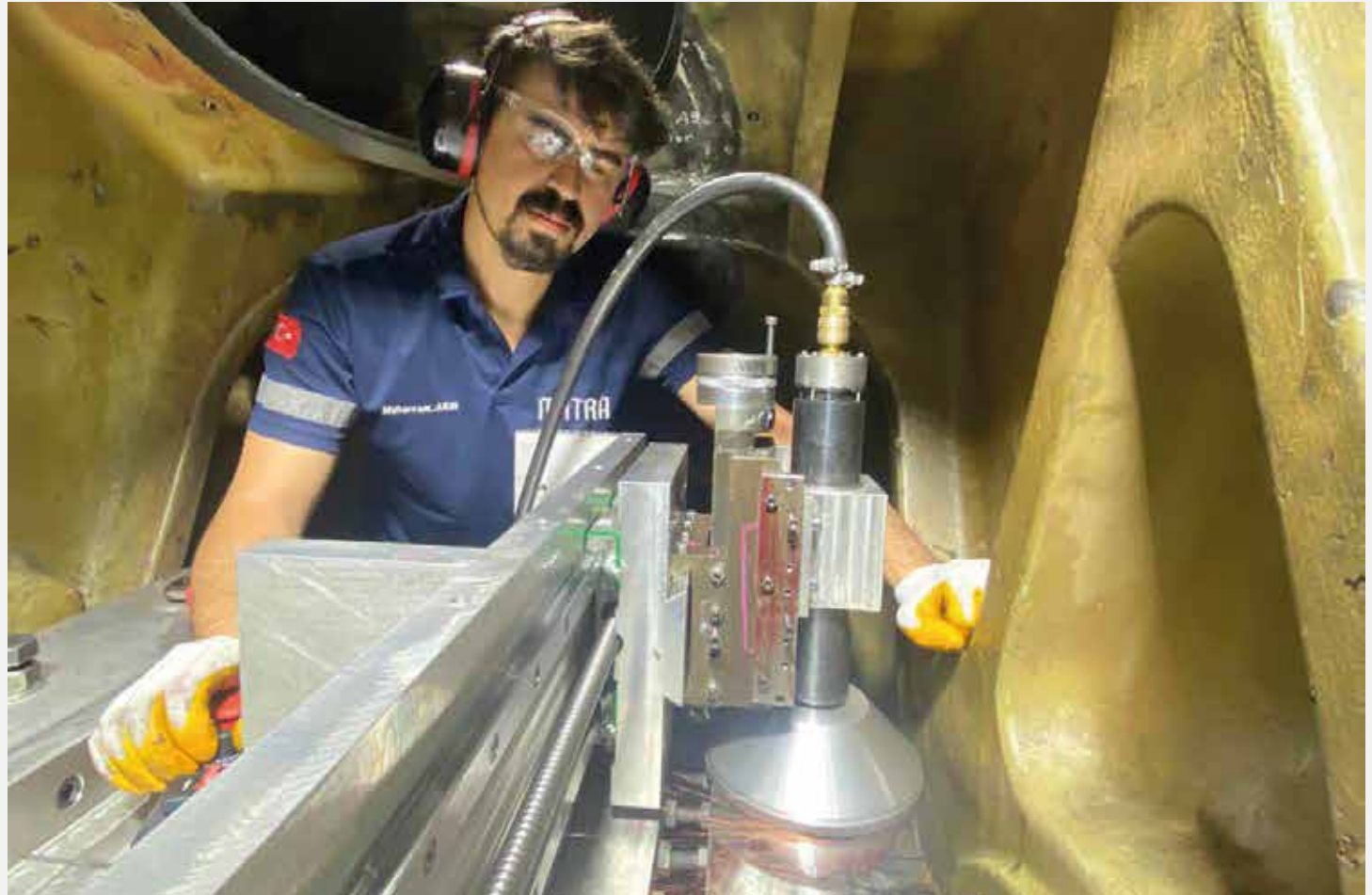
Surface Grinding of Counterweight Contact Surface
