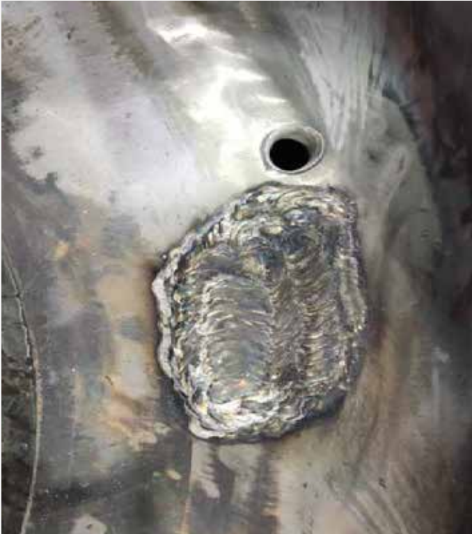
Inconel 625 Welding Around Injector Holes
