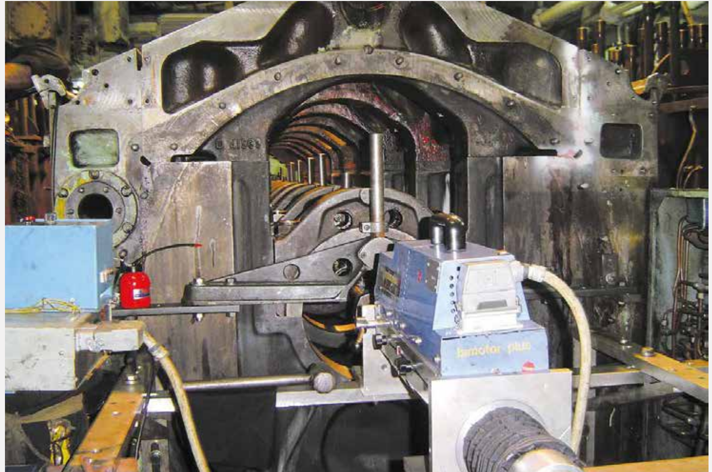
Line Boring of Main Bearing Journals in the Engine Room
