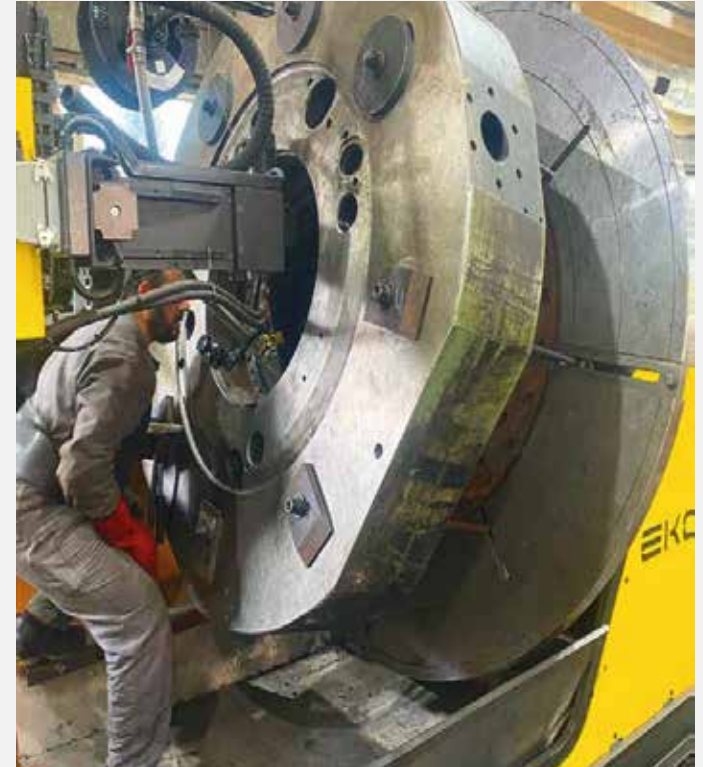
Welding of 90MC Cylinder Head
