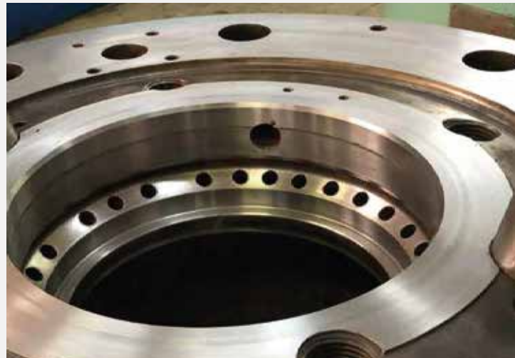
Reconditioning of Cylinder Heads by SAW and CNC Machining
