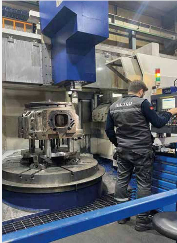
CNC Machining of Cylinder Head Sealing Surfaces
