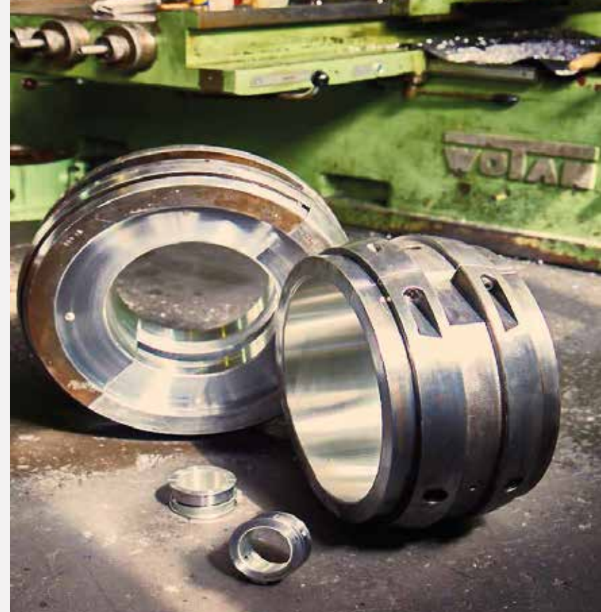
Repaired Alternator Shaft Bearings
