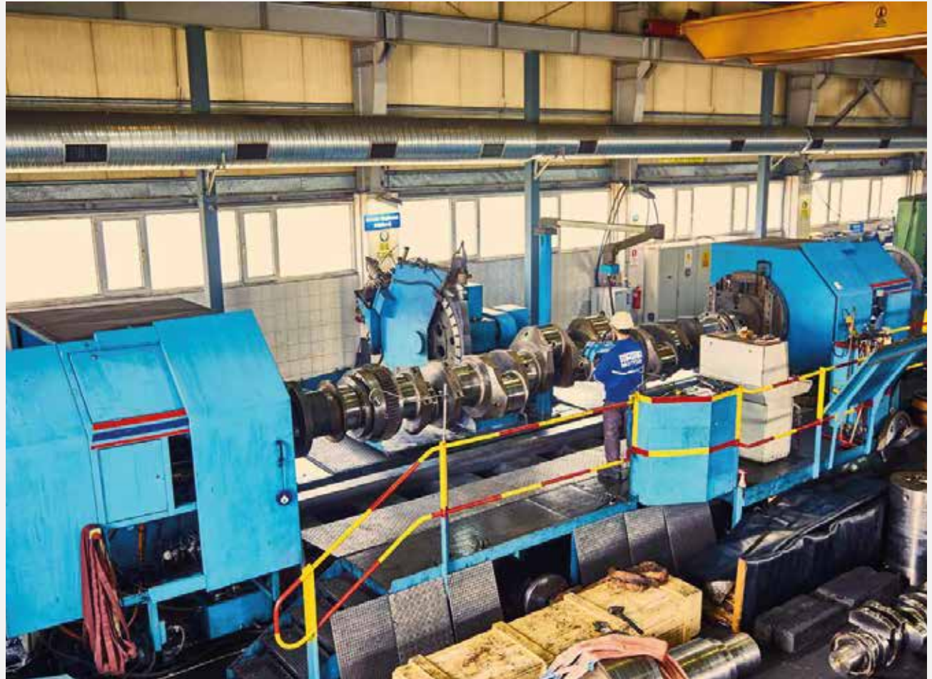
Crankshaft Grinding of Wartsila 46 - 6500mm long & weighs 10 tons
